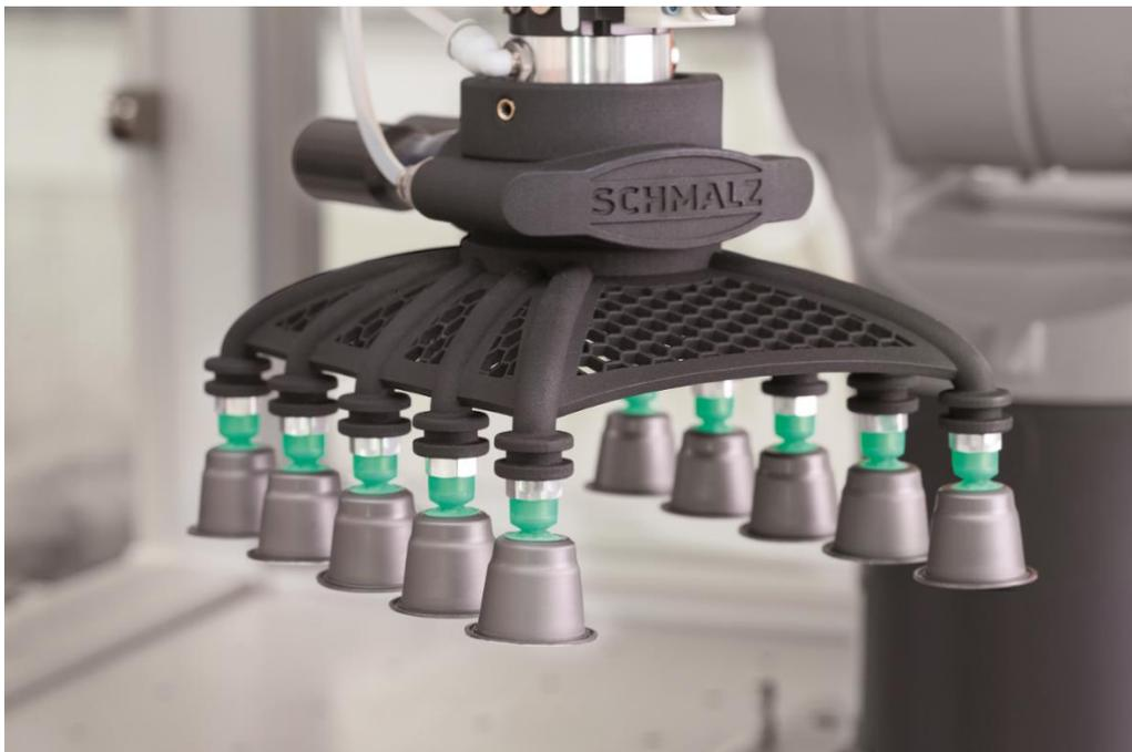
*Robotics grippers from Schmalz can be designed for specific applications and manufactured additively using trinckle software. Copyright: Schmalz*
