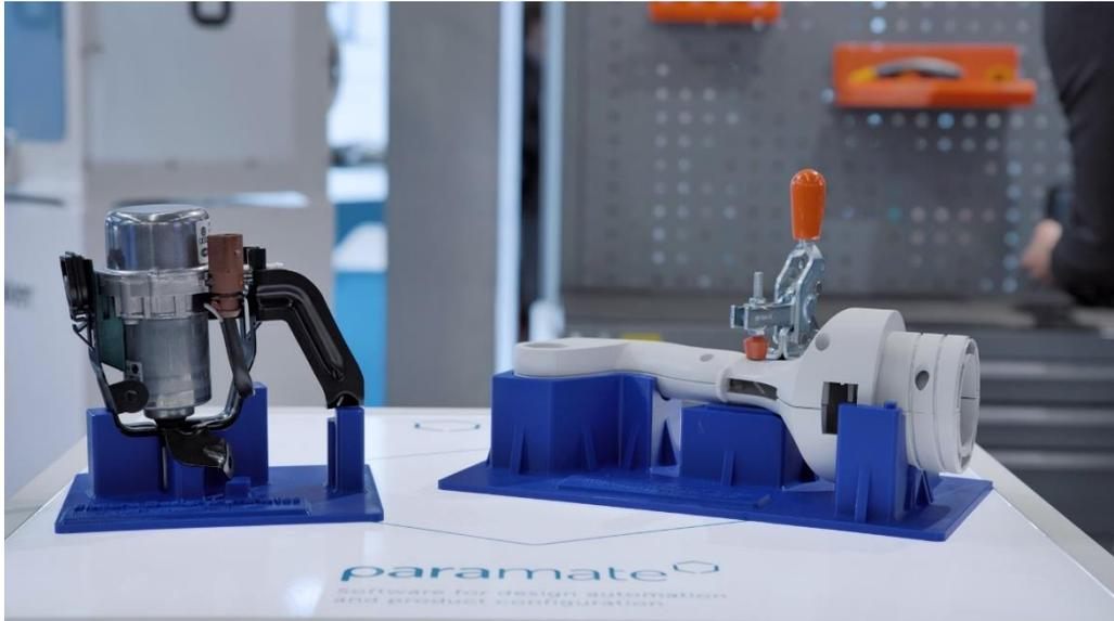
*Assembly and measuring fixtures can be easily designed in trinckle software and additively manufactured at low cost. Copyright: Ultimaker, trinckle*
